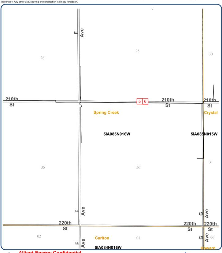
indefinitely. Any other use, copying or reproduction is strictly forbidden. 25 210th St **Spring Creek** 5IA085N016W 36 Install a span of undergorund cable. Install an anchor 12' E of #5 and 12' W of #6. Retire a span of conductor.
